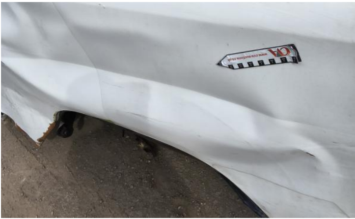
3: Door osf Dented With Paint Damage
