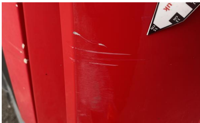
10: B Post ns Dented Over 30mm
