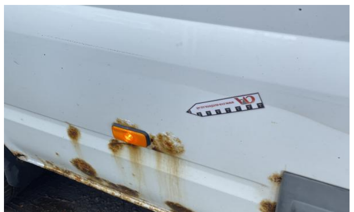
6: Qtr Panel osr Rusted Over 5mm
