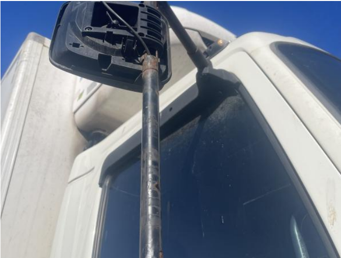
4: Door Mirror Assy osf Broken Replace
