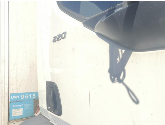
5: Door osf Dented With Paint Damage
