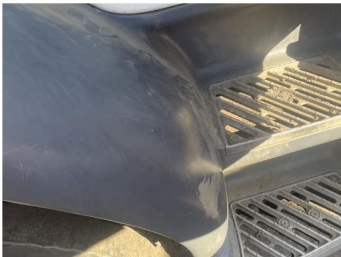
1: Door Moulding of Scuffed (Unpainted) Over 100mm
