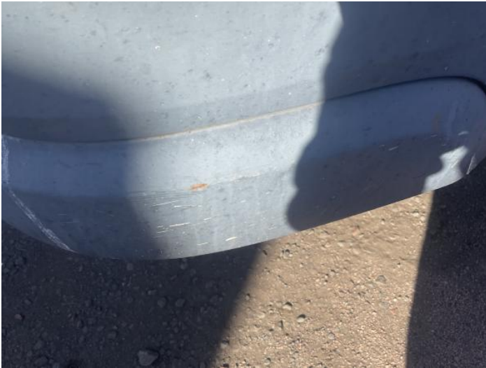
3: Bumper Front Moulding Scuffed (Unpainted) Over 100mm
