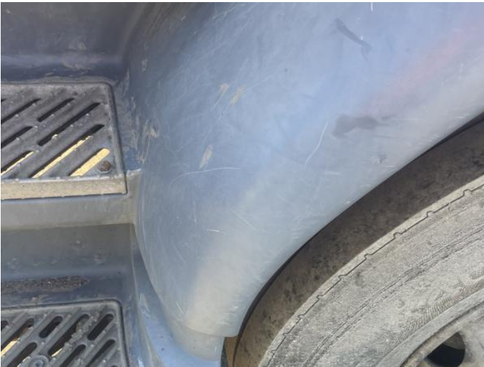
6: Door Moulding nsf Scuffed (Unpainted) Over 100mm
